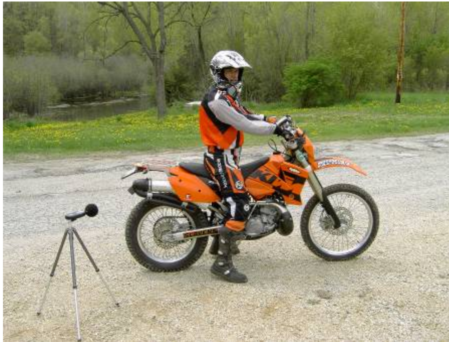
Exhibit 1: Stationary Motorcycle Exhaust Noise Measurement
